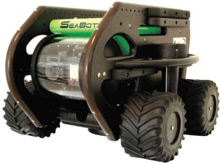
This is how the newly developed subsea vehicle looks like. The skid with a four-wheel drive enables the crawler to perform inspections with a stability that a conventional ROV cannot achieve.
