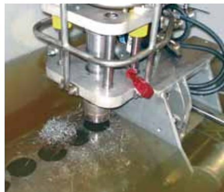
The special Imenco-designed drilling rigs were tested under water before delivery to the customer.
